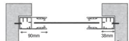
Undersize fix (Where some of the guide track will be into the opening)
