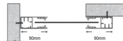
Combination of face fix and reveal fix
