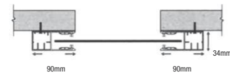
Face fix (Fixing behind the opening)
